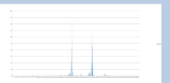
Spectrum collected by RaMonA by drawing air from the ground. The 222Rn and 220Rn  $\alpha$ - lines can be observed. The main peculiarity of the system is the possibility to separate, thanks to  $\alpha$ -spectroscopy, the two most abundant isotopes of radon. The energy resolution is 20 keV
