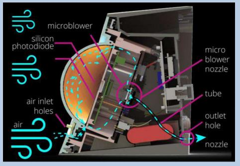
The amount of radon entering a measuring chamber, either by diffusion or transported by an air stream, is monitored by detecting the alpha particles emitted by the radioisotope's descendants. This detection technique is the only one that allows the independent observation also of the 220 isotope of radon, called thoron.
